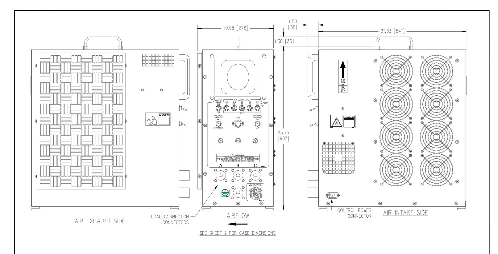
3. UNIT IS SUPPLIED WITH 10" [3m] LONG LOAD CONNECTION CABLES AND 115V POWER CABLE.
